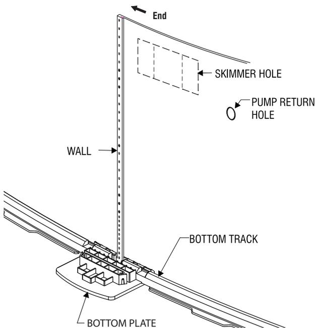
Once the wall is completely uncoiled, you may find that it is too long or that both ends do not meet by a few centimetres. If such is the case, adjust tracks and joiner plates until wall holes line up. If this does not work, roll up the wall again, check measurements as per Illustration 1.1, adjust tracks and plates, if applicable, and uncoil the wall again. If the spread is too wide, measure the wall and check it against the chart below.
