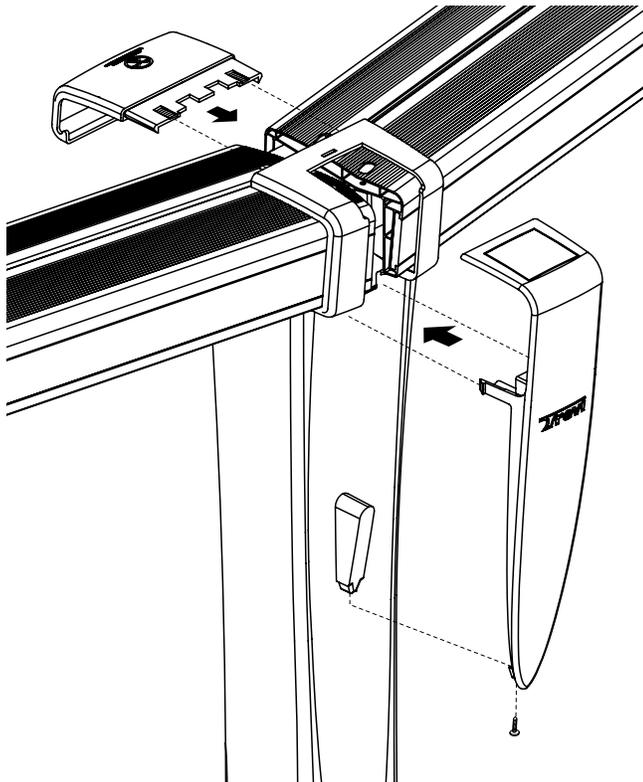
Put the seat cap on the inside section of the seat and interlock with the upright. Secure the seat cap with one (1) screw "Z".
