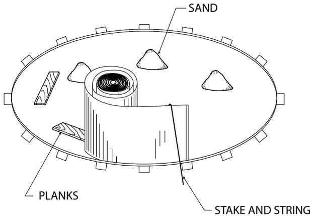
Begin inserting the wall into the bottom wall tracks in the middle of a joiner plate. At first, the wall is kept in place with one or two stakes and strings (or extra persons). One person uncoils the wall on a beam or a plank, while a second person inserts it in the bottom wall tracks. Do not uncoil more than 3 m (10') of wall before you install a support bar or stake and string to reinforce the structure.
