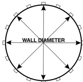
Make a complete circle, using half of the wall tracks and joiner plates found in the pool kit (See Chart and Illustration 4.2).
