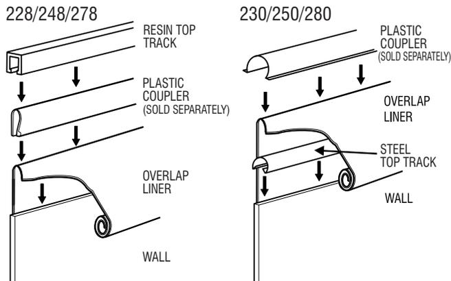
Installation detail of a bead liner with top track. Hang the liner on the top of the wall and install the top track to secure.
