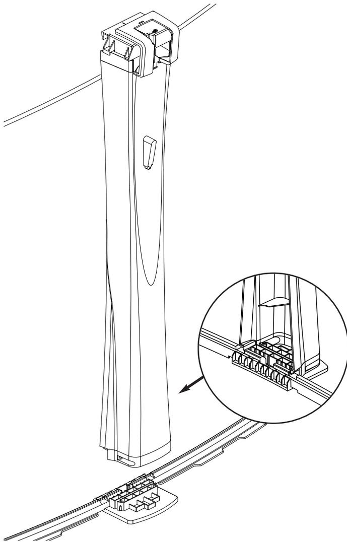
Attach the uprights to the bottom plate with two (2) screws "Z", which you will find in the hardware bag.
